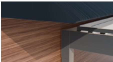
Additional clearance required above the post height
